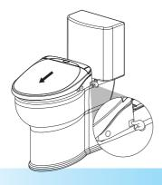
③ Press fast-install button. Remove the cover seat from toilet.
