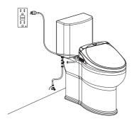
① Unplug the product and turn off the shutoff valve. Remove the braided hose and drain excess water.
